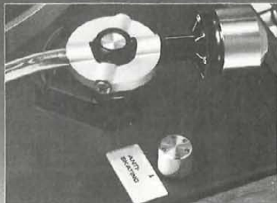
Anti-skating control insures perfect tracking.
